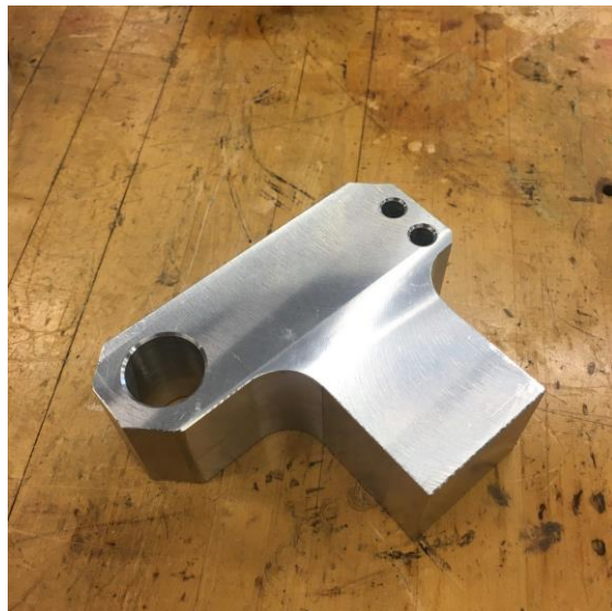
Figure 24. Angling mechanism to adjust rail angle
