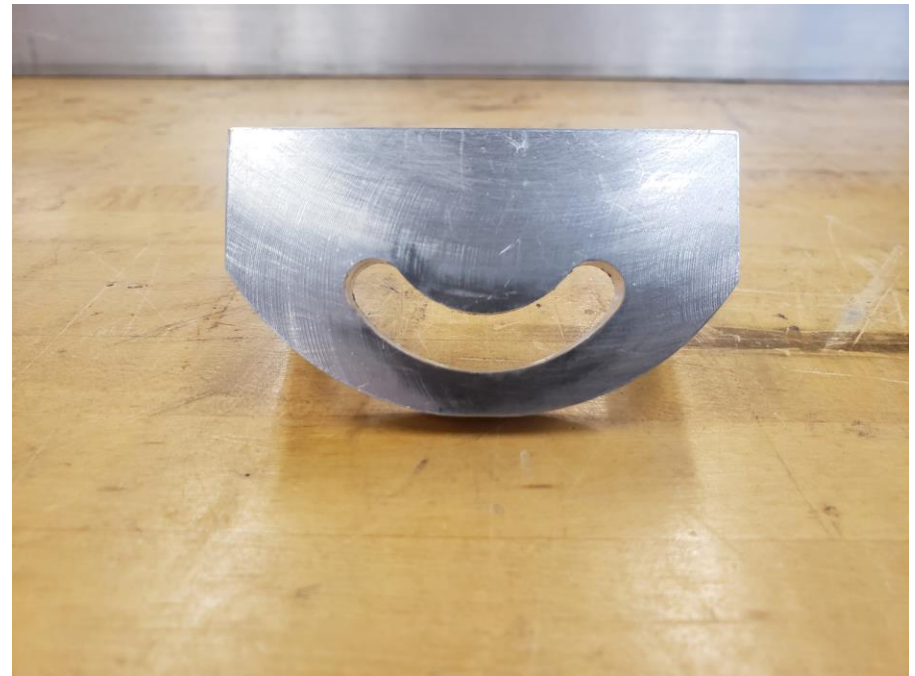
Figure 23. Angle positioner for template holder
